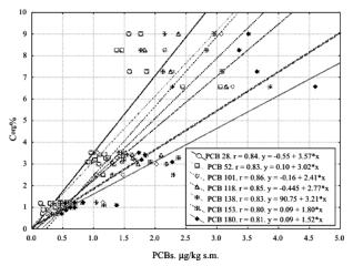
Fig. 2. Relationship between the PCBs concentration and content of organic carbon ( $C_{org}$ ) in bottom sediments.
